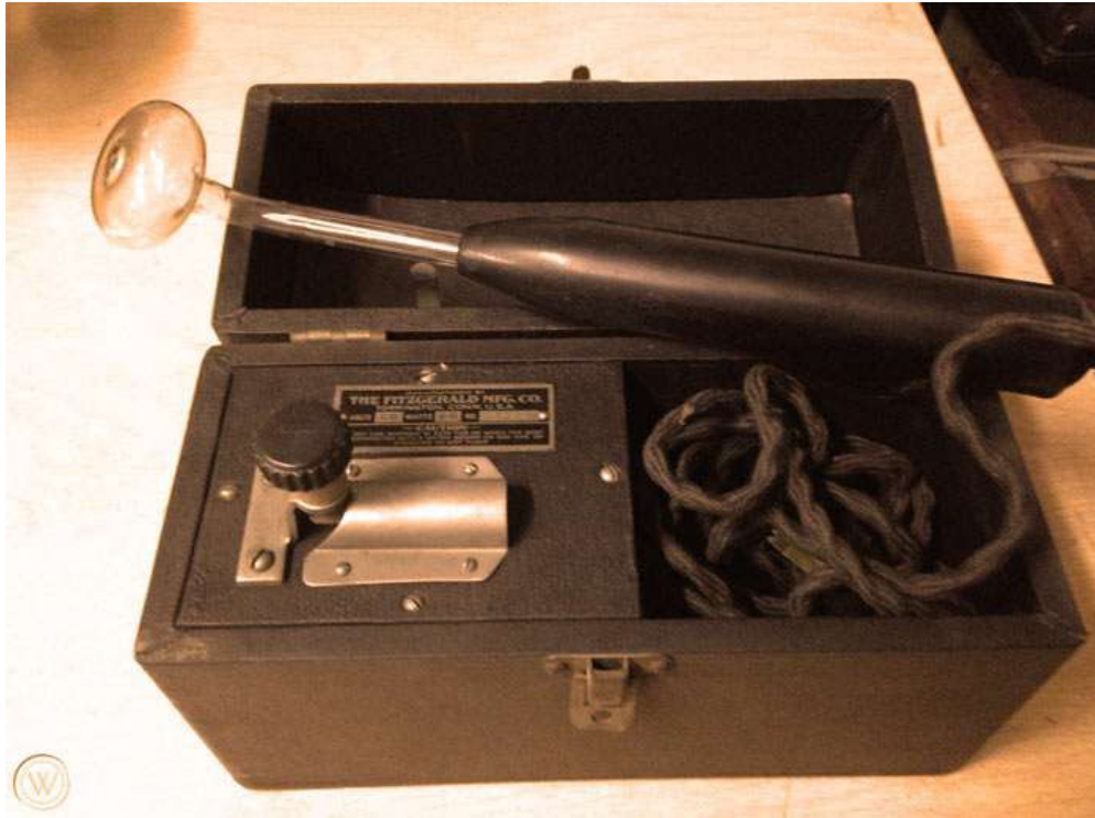
Vintage Electrotherapy Violet Ray, made by Fitzgerald Manufacturing Co., Torrington, CT, ca. 1926. The low frequency coil is in the box inside the case. It is connected with a wire to the high frequency coil inside the handle with the glass electrode.
